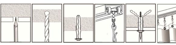
Using the Track as Pattern, Mark Holes on Ceiling
